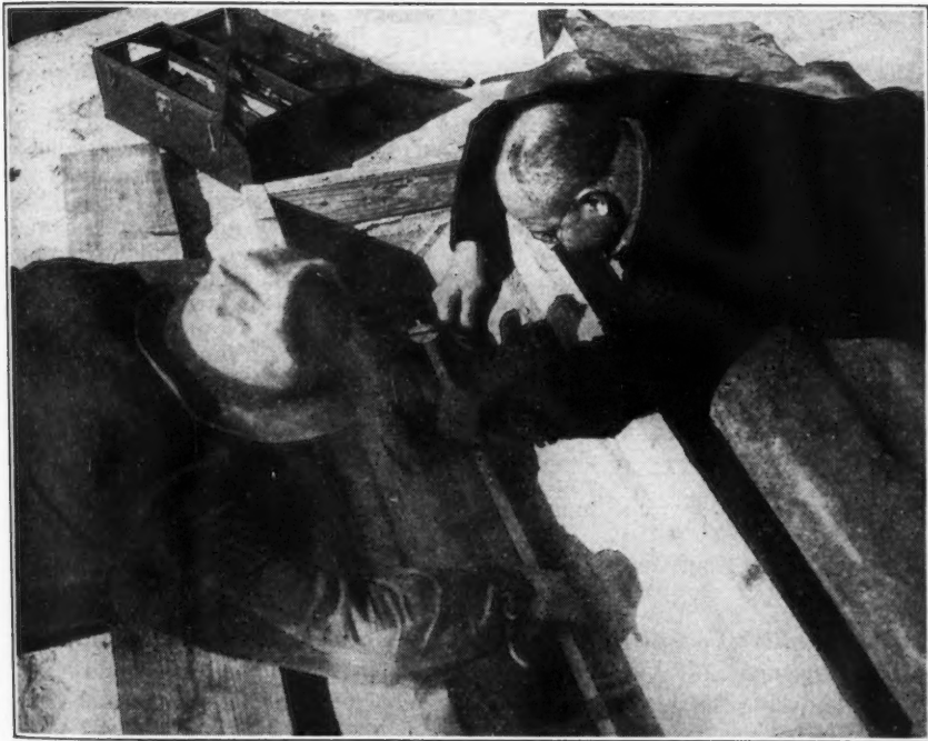
FIG. 5.—MAKING STRAIN-GAGE MEASUREMENTS WITH SPECIAL EXTENSOMETER
